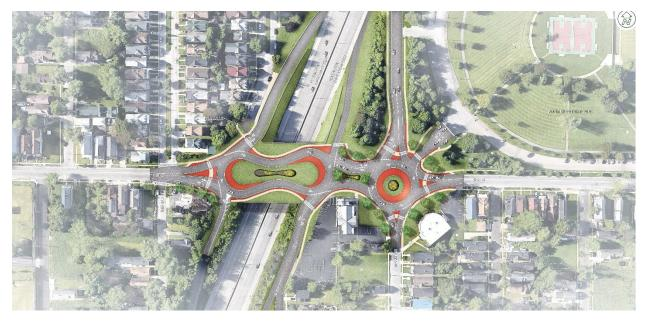
Figure 3: Plan of Best Street crossing and roundabout under the Build Alternative between Wohlers Avenue and Rich Street.
